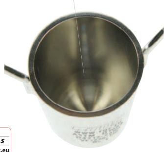
STANDARDS ASTM D1084 ASTM D4212
