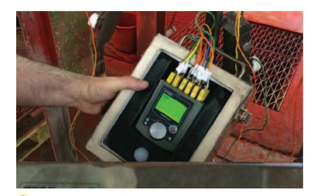
The temperature of the different areas of curing ovens can be separately adjusted. However, it is not easy to identify whether the temperature of the product itself and the exposure time will produce the desired results. In the case of powder coatings, if the curing time is too short or the temperature too low, the coating will not crosslink properly.
